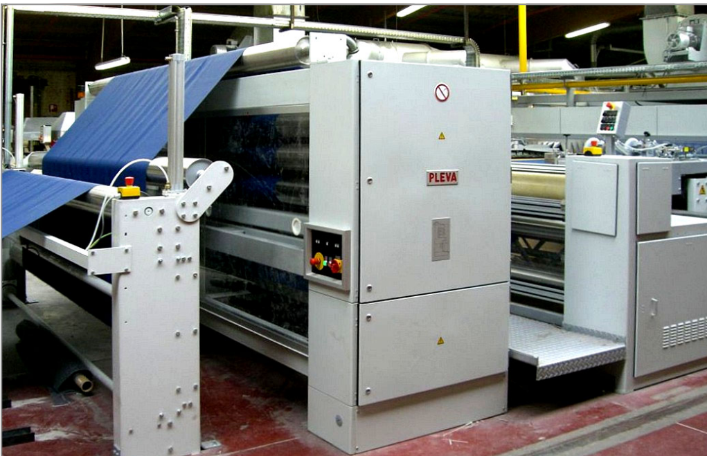
Picture 1: Installation of advanced PLEVA StraightLiner with traversing camera in front of stenter frame.
