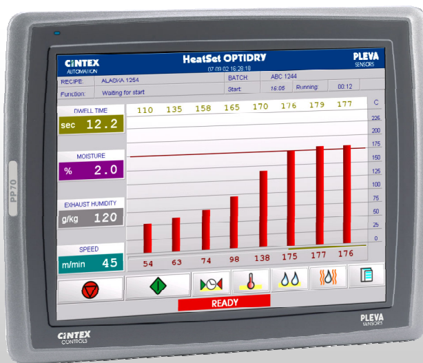
CINTEX-PLEVA control panel with touch screen and OPTIDRY "Auto-Setting" function.
